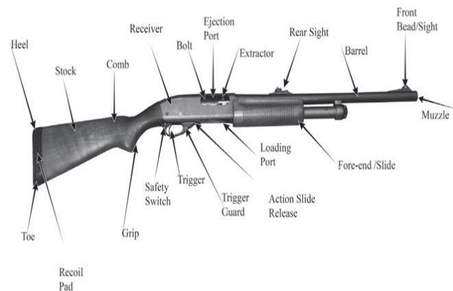
(Figure 2-5) Shotgun pump action nomenclature Position of parts may vary depending upon the make and model of the weapon.
